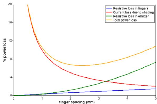
Next, focus in on the two key adjustable parameters for this activity: Finger spacing ( $S_f$ ) and busbar spacing/finger length ( $L$ ). Show two different front grid designs. Ask two questions:
