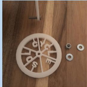
3b. Add [washer - wheel - washer] and then tighten on the lock nut. The wheel should still spin freely. If it does not, remove one or both of the washers. If there is too much room on the screw and the wheel wiggles, add another washer.
