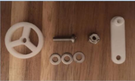
2a. Add [washer(s) - wheel - washer(s)] to the bolt, so that there are washers on either side of the wheel.
