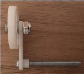
4b. Add the [lock washer - nut], then screw bolt into the bicycle frame. This training wheel should be on the opposite side of the protruding top bar, on the opposite side of the front wheel.
