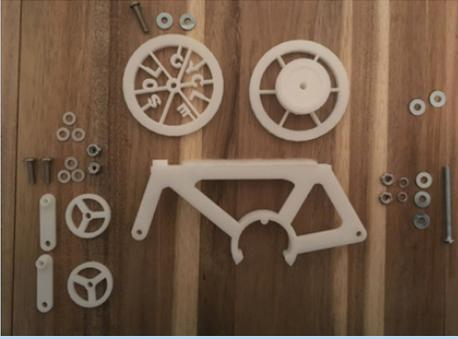
2. Assemble the training wheels (x2) The number of washers you need will depend on the thickness of your washer – they are there to help your wheel spin, and also to make sure the screw fits snugly into the lock nut. Follow these steps for both training wheels.
