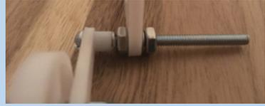
4d. Add a [washer], then carefully tighten on the other training wheel by lightly pressing the opening of the nub against the end of the bolt. It should turn 3-5 times but can easily break if you apply too much pressure.
