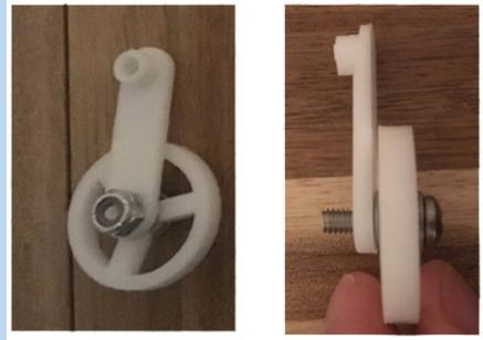
3a. Front wheel. Screw the bolt into the front wheel slot. You may need a screwdriver to do this. The head of the bolt should be on the opposite side of the protruding top bar (the same side as the flat face), so the front and back wheel will align.
