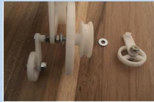
5. Finishing touches: it is pretty tricky to get those back wheels to stay in place. The easiest way to do it is to make sure the training wheels are aligned and touching the ground, the nut on the opposite side of the back wheel is tightened all the way up against the training wheel, and then use pliers to tighten the nut closest to the back wheel. Play around with it.
