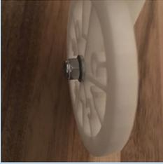
4a. For back wheel, twist the training wheel with the open hole onto the long (1.75 or 2" screw) with the nub facing in and the wheel facing out as shown.
