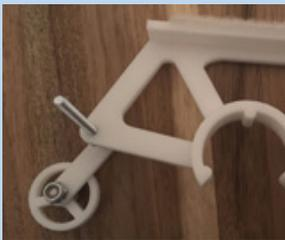
4c. Add [lock washer - nut - washer] as shown. Then add on the back wheel, with the pulley-side of the back wheel facing away from the frame.
